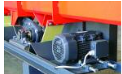
Vibrating conveyor system with integrated drive train
