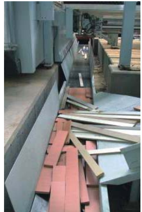
Leopard 600 in an angular saw application fed with a vibrating conveyor
