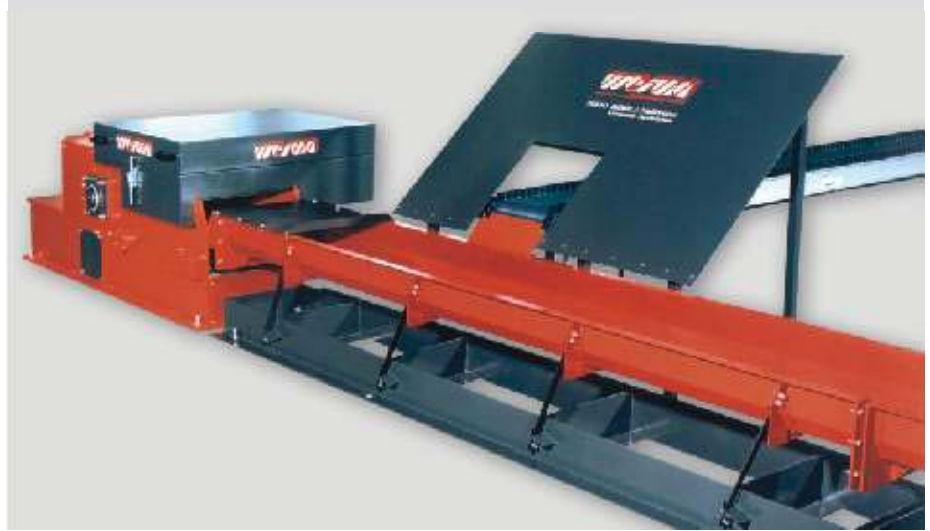
Leopard 800 with combined feeding system for blocks and strips integrated in a fully automatic roughmill application
