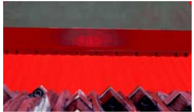
cutting chamber with WING-RAM and WEIMA-V-Rotor
