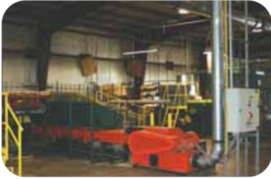
A Weima Tiger horizontal shredder reduces scrap edgings from the saw and feeds the waste into the central dust collection system.
